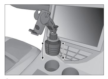
Place the device on the two pads. Press the two arms inward to secure the device. To release the device push the release button on the bottom.
